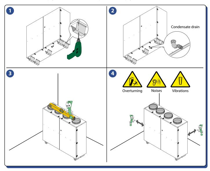
3. Place the unit on the floor and check levelling with the aid of a spirit level: the unit must be installed perfectly flat to ensure proper drainage of condensation water.
